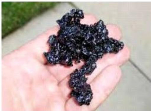
Prior to placement TBTRA has a sticky appearance resulting from mixing a liquefied tire rubber blend with aggregate.
